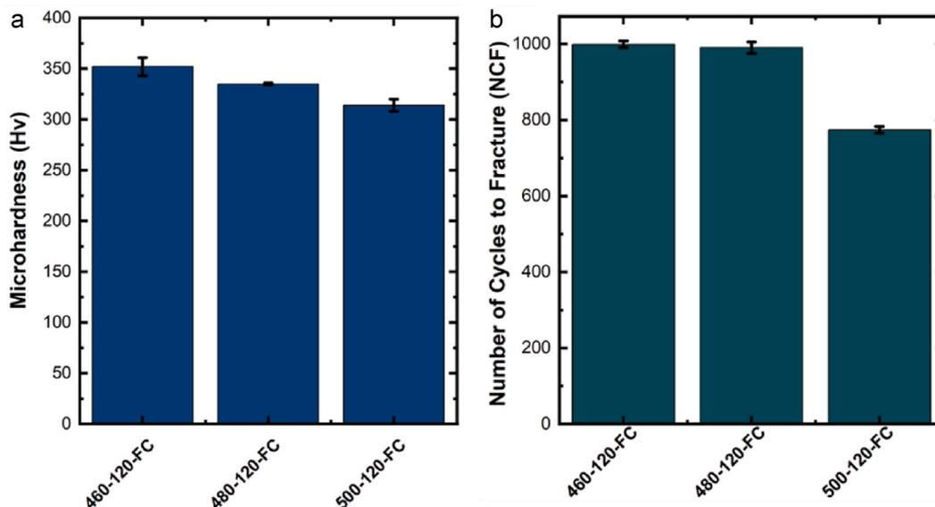
**Fig. 6.** a) Vickers microhardness values and b) number of cycles to fracture (NCF) after rotary bending tests of heat-treated NiTi rotary files at 460, 480, and 500 °C for 120 min.
