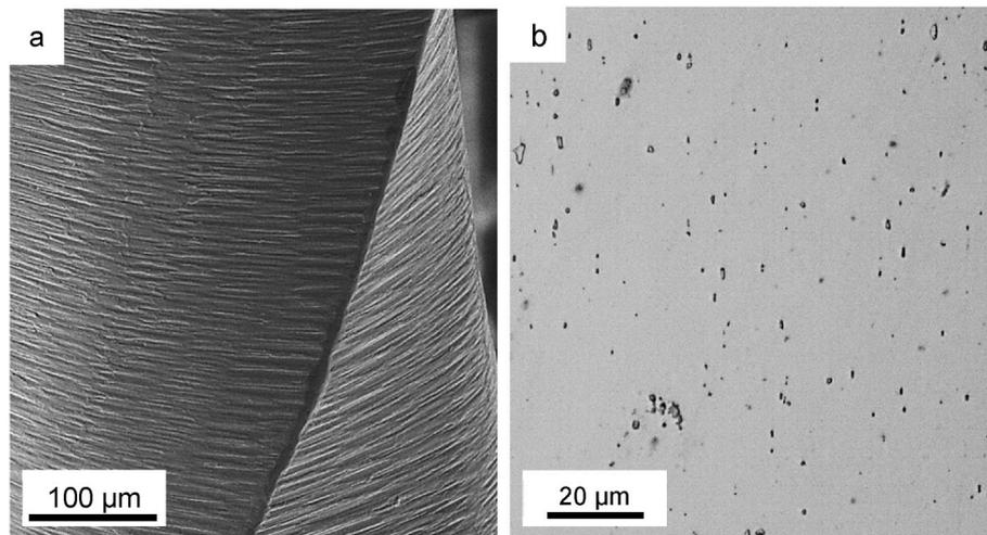
Fig. 2. (a) SEM micrograph showing the surface topography and (b) optical microscopy image of the longitudinal cross-section of the rotary file.
