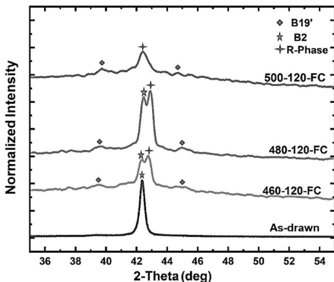
**Fig. 5.** X-ray diffraction patterns of NiTi rotary files before and after heat treatment at 460, 480 and 500 °C for 120 min followed by furnace cooling.
