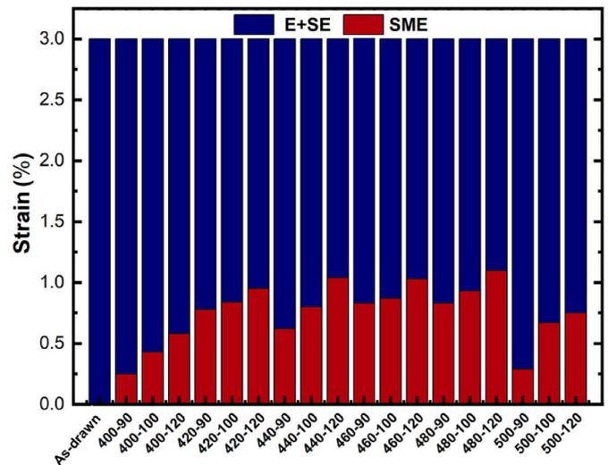
Fig. 3. Recovered bending strain (E + SE and SME) of NiTi rotary files before and after heat treatment at 400, 420, 440, 460, 480 and  $500^\circ C$  for 90, 100, and 120 min followed by air cooling.
