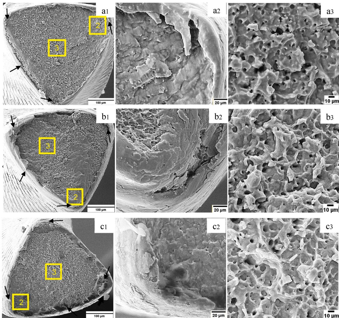
**Fig. 7.** SEM micrographs of fracture surfaces of heat-treated NiTi rotary files at a) 460, b) 480 and c) 500 °C for 120 min. Black arrows show crack initiation sites, and areas labeled by 2 and 3 represent crack propagation and final fracture areas, respectively.
