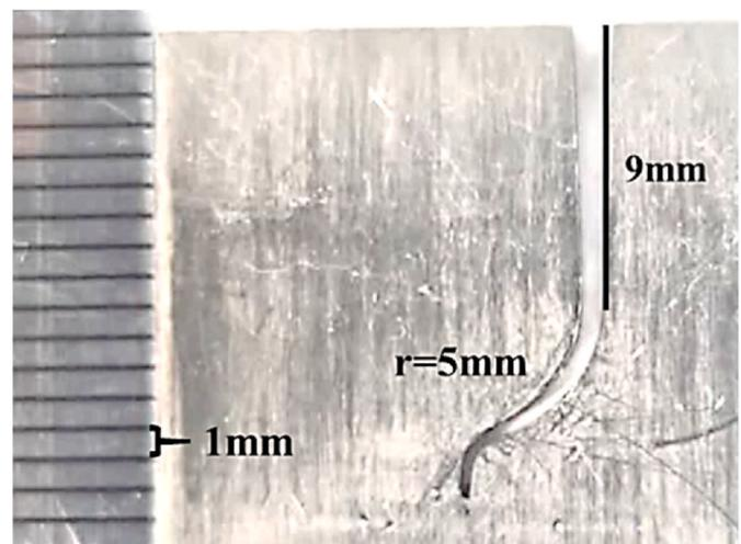
Fig. 1. Simulated root canal in a steel block used for cyclic rotary bending fatigue tests, illustrating a curvature radius of 5 mm.
