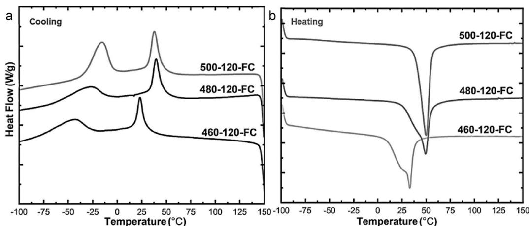
Fig. 4. DSC curves at (a) cooling and (b) heating regims for heat treated samples at 460, 480 and 500 °C for 120 min followed by furnace cooling.
